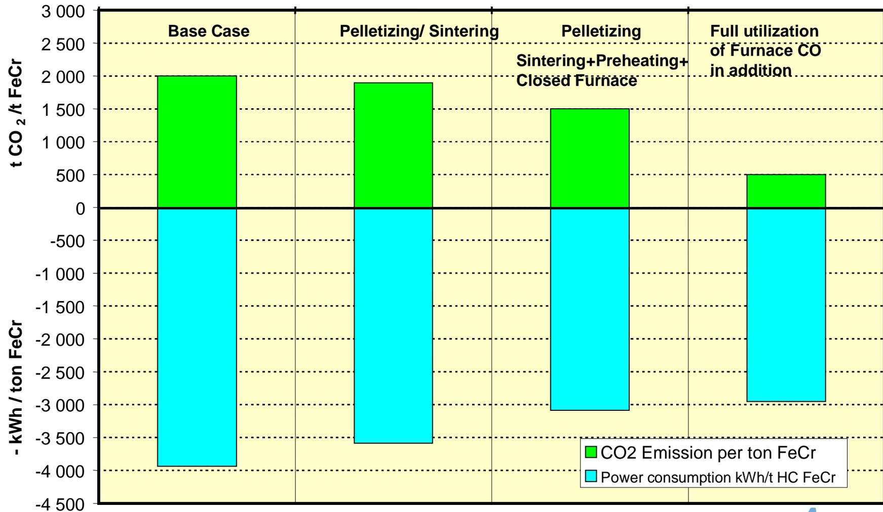
Without technology development the CO<sub>2</sub> emission level at Outokumpu Tornio FeCr plant would be more than 3-fold compared to the present actual figures
